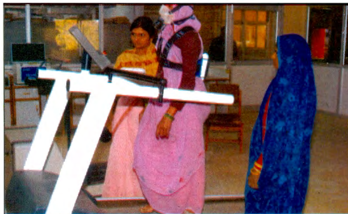
Plate 5 : Measurement of Heart rate and oxygen consumption of farm women on tread mill using metamax ambulatory metabolic measurement systems
