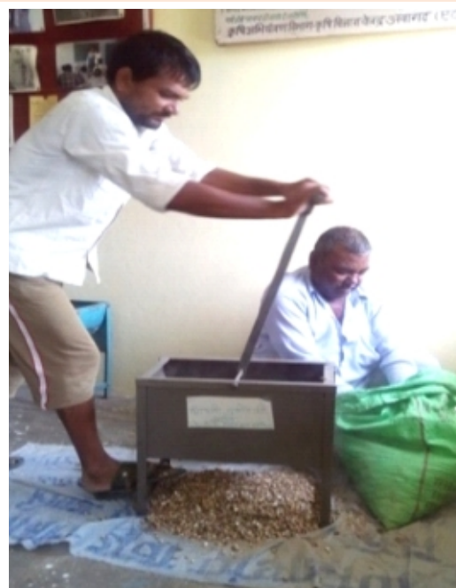
Inclined concave opening (Refined Groundnut decorticator)
