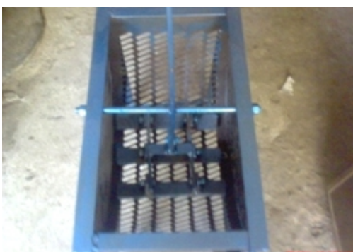
Inclined concave opening (Refined Groundnut decorticator)
