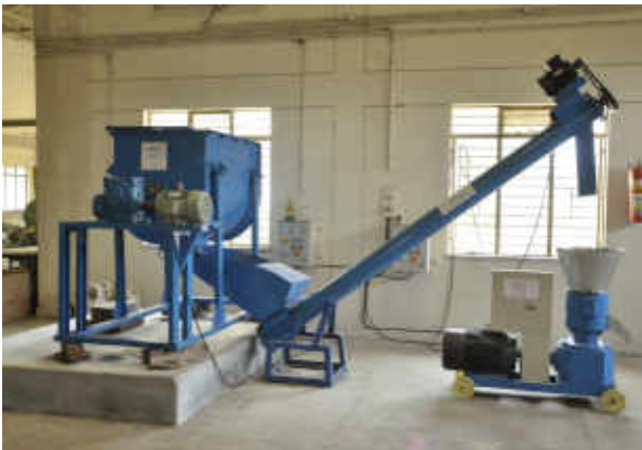
Cotton stalk pelletizing unit installed at GTC, Nagpur
