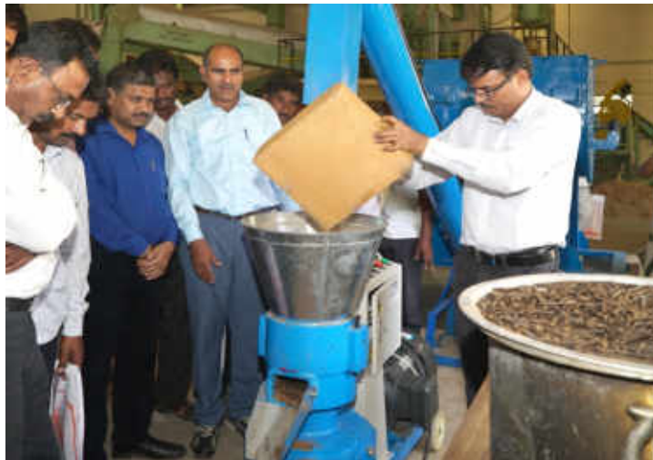
Fig. 3.10 Demonstration of Pelletising machine for converting cotton stalks into pellets at Technology and Machinery Demonstration Mela on March 21, 2016 at GTC, Nagpur
