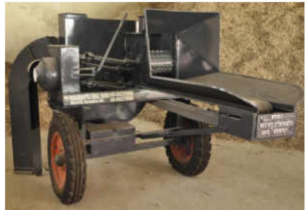
Cotton stalk chipping unit installed at GTC Nagpur
