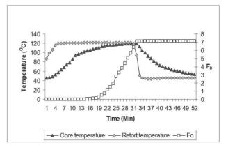
Fig. 5. Heat penetration characteristics with respect to  $F_0$  of crab koftha processed to  $F_0$  7 in TFS can
