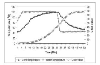
Fig. 6. Heat penetration characteristics with respect to cook value of crab koftha processed to  $F_0$ 7 in TFS can
