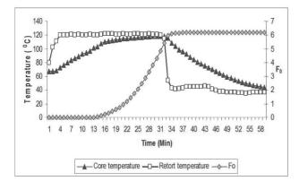
Fig. 3. Heat penetration characteristics with respect to  $F_0$  of crab koftha processed to  $F_0$  6 in TFS can
