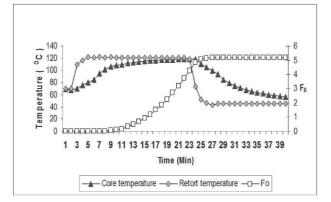
Fig. 1. Heat penetration characteristics with respect to  $F_0$  of crab koftha processed to  $F_0$  5 in TFS can
