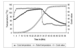
Fig. 4. Heat penetration characteristics with respect to cook value of crab koftha processed to F<sub>0</sub> 6 in TFS can
