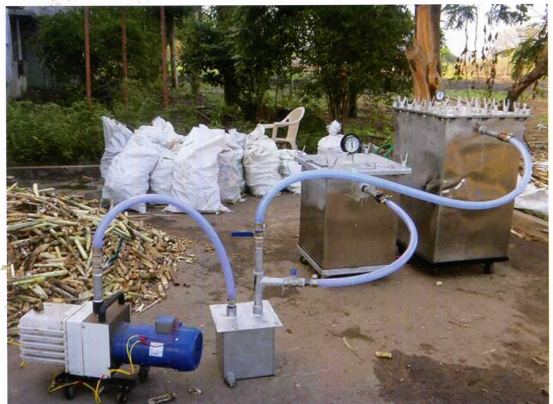
Sett treatment devices are in operation for effective treatment of fungicides in sugarcane setts to manage red rot and smut.
