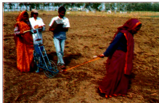
Force measurement during operation of PAU seed drill
