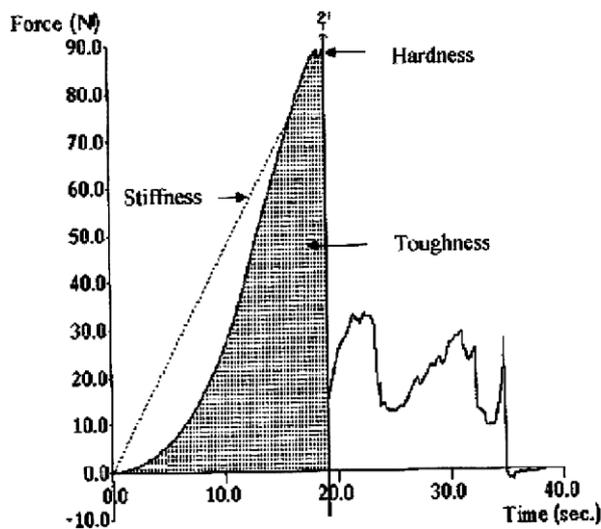
Fig. 2. Typical force-time deformation curves during compression/penetration for *Rohu* fish.
