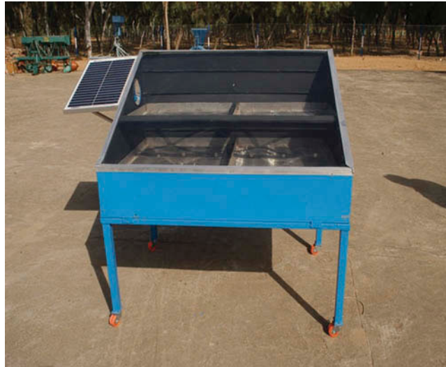
Figure 3. PVT hybrid solar dryer installed at CAZRI solar yard.
