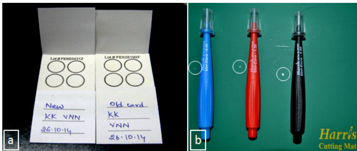
Figure 1: FTA Elute Card for sample application (a) and the Harris Micro Punch (b) for cutting disc dimension of 0.5, 1.2 and 2 mm diameter (note the encircled area).
