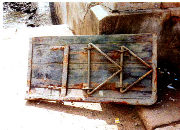
Fig. 2. Wooden otter boards used in Vengurla
