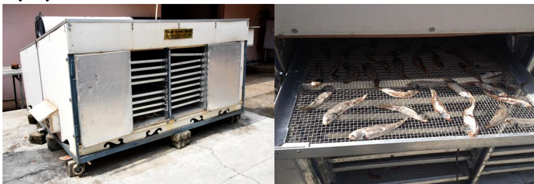
Fig.5. CIFT Solar-Cabinet Dryer with Electrical back-up
