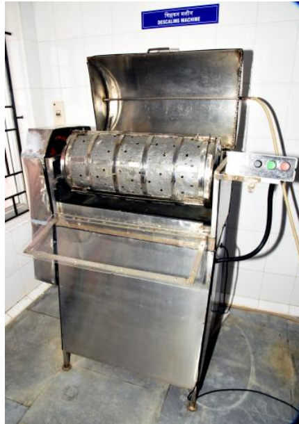
Fig.6 Fish de-scaling machine with variable drum speed
