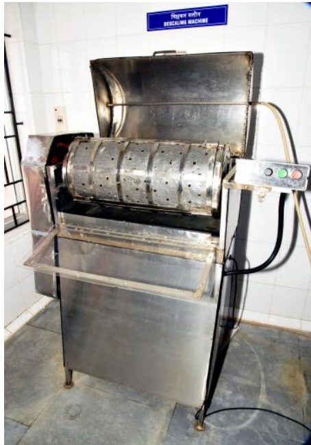
Fig.6 Fish de-scaling machine with variable drum speed
