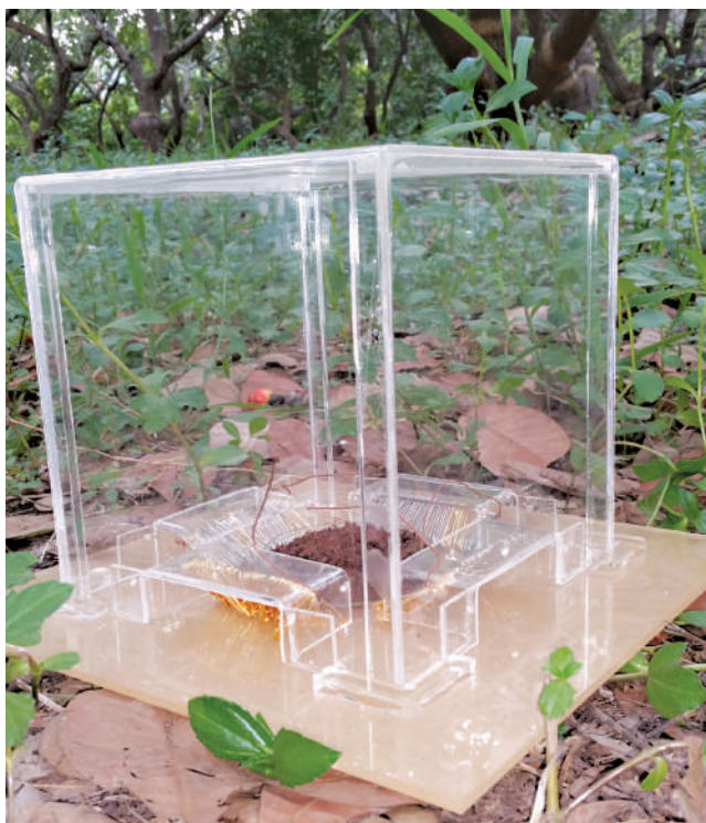
Fig. 3.3.2. Physical traps designed for evaluating kairomone blends for CSRB
