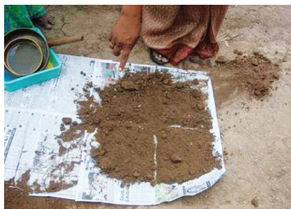
Fig. 4. Quartering for reducing sample volume while mixing the composite samples
