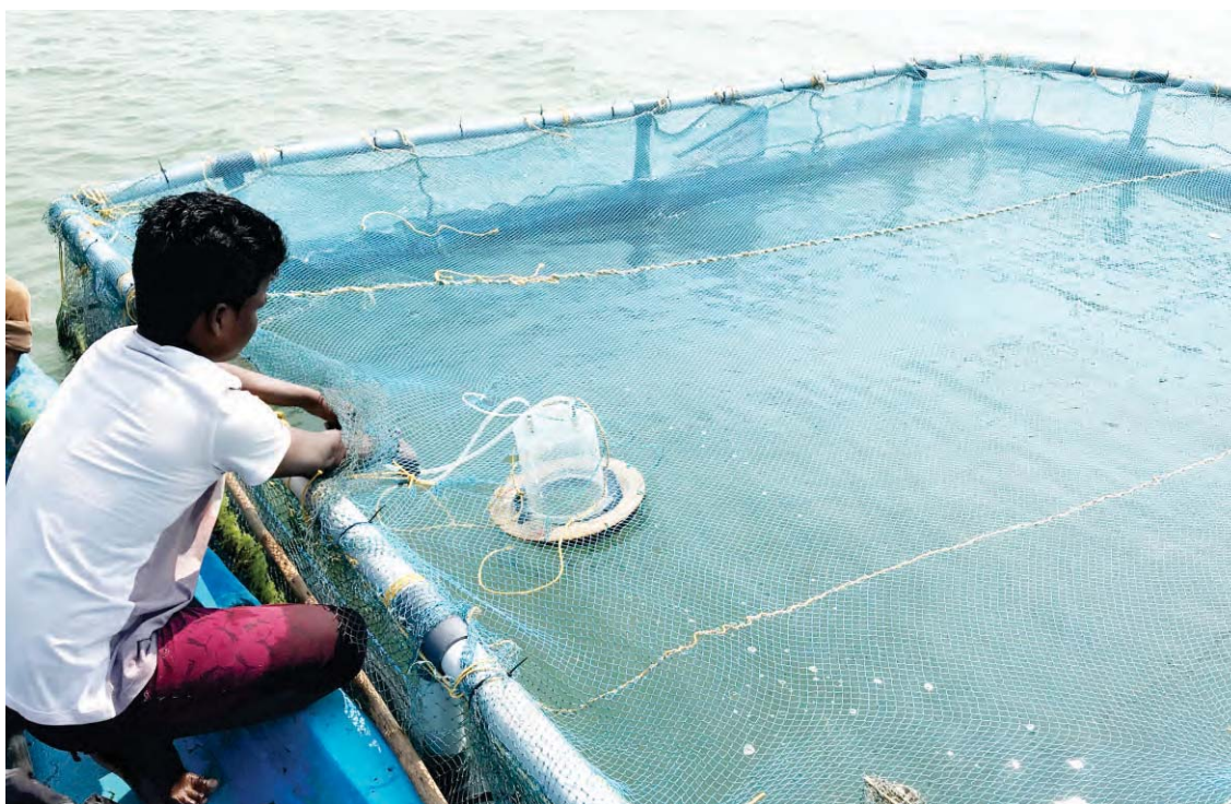
Collection of GHGs from Seabass cage culture systems installed in open waters at Venangapattu, Tamil Nadu
