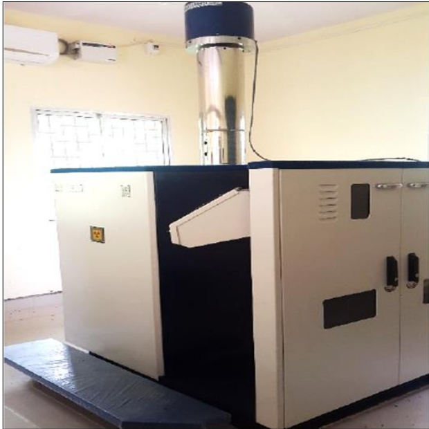
Plate 1: View of gamma chamber used for induction of mutation in papaya
