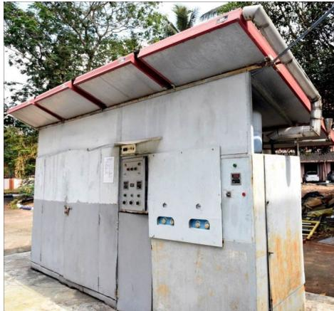
Fig.1. CIFT Solar-LPG Dryer
