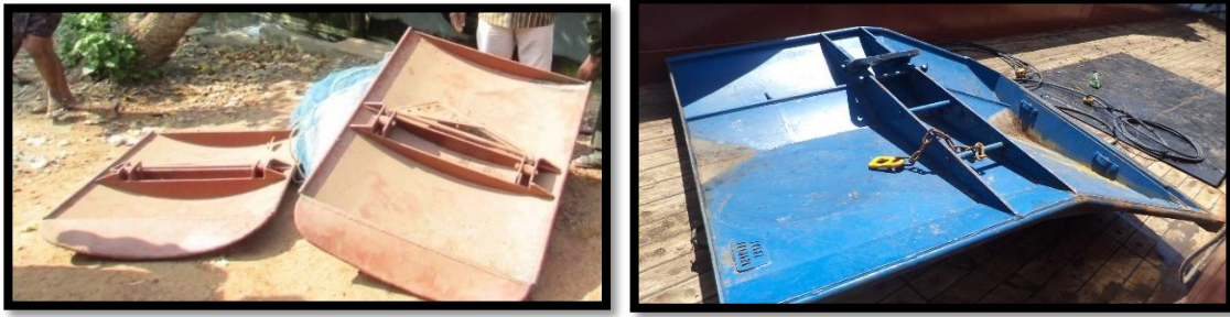
Fig.8. Suberkrub otterboards and Thyboron type-7 otterboard
