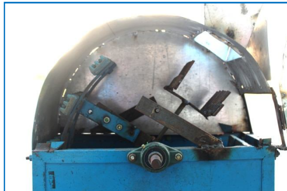
Arrangemet of Decortivating and Stripping shoes
