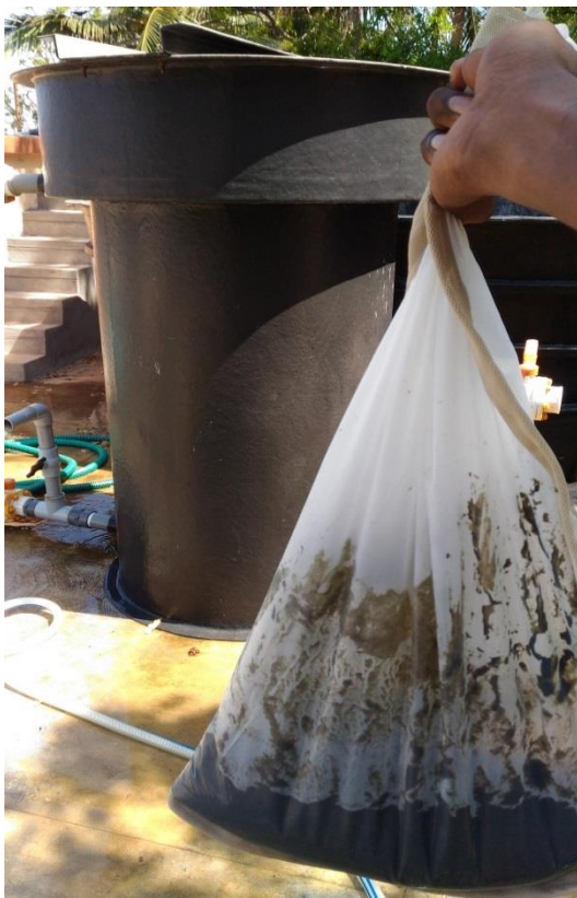
Fig 2. Harvesting of bioflocs using radial settler
