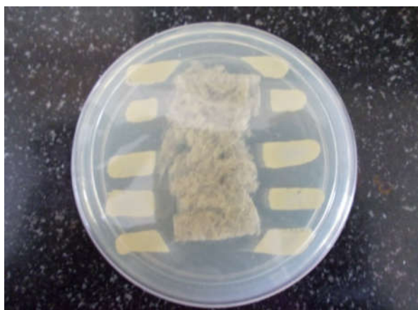
Fig. 2 Presence of zone of inhibition on treated Samples (AATCC 147)
