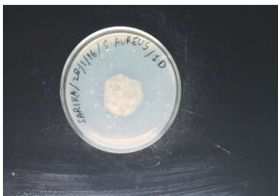
Fig. 1 Presence of zone of inhibition on treated Samples (ENISO 20645)
