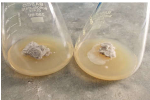
Fig. 3 Treated sample showing no fungal growth and test control (ENISO 20645)
