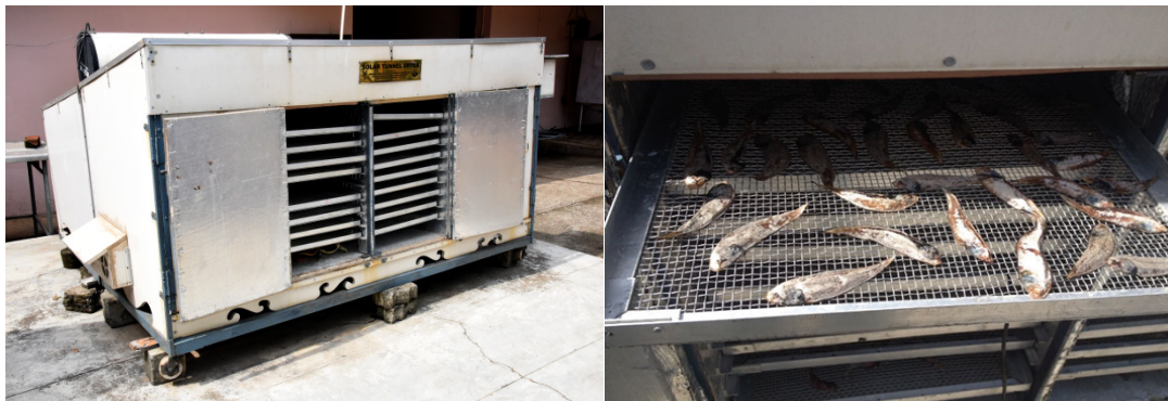
Fig. 5. ICAR-CIFT Solar-Cabinet Dryer with Electrical back-up
