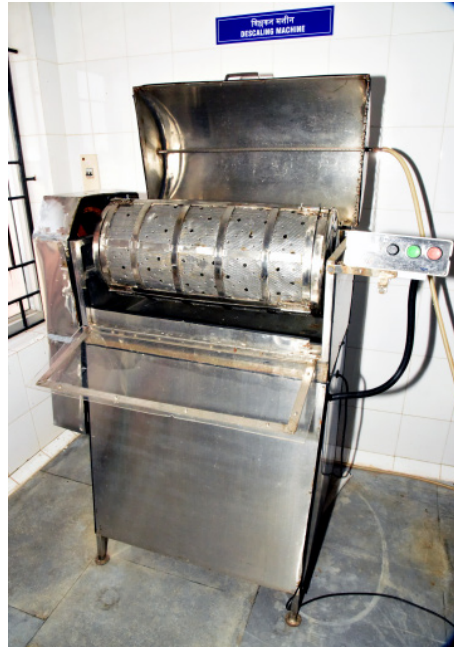
Fig. 6. Fish descaling machine with variable drum speed
