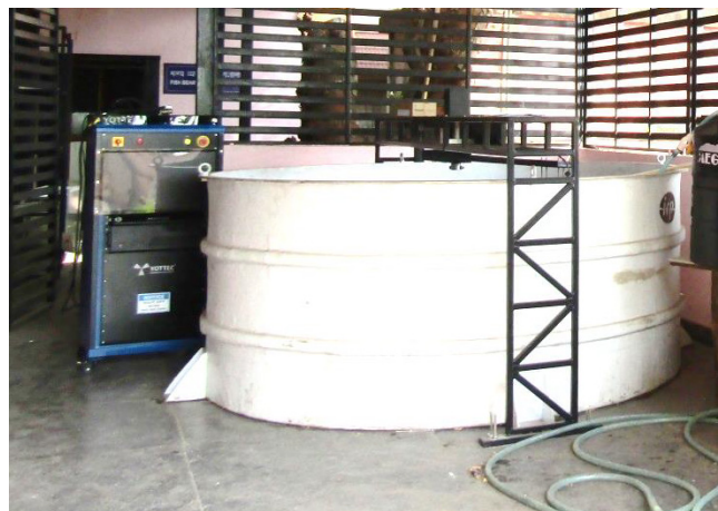
Fig. 3 Moving gantry system installed at ICAR-CIFT for studying swimming speed of fish
