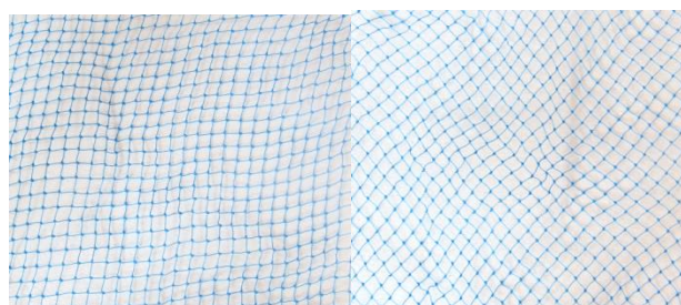
Fig. 5. Square and diamond shaped HDPE webbing
