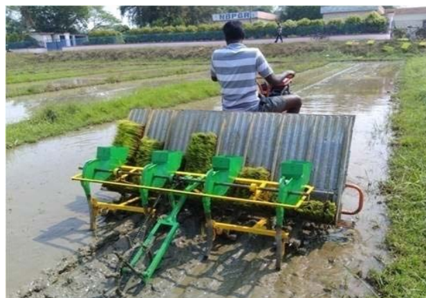
Fig. 2.10. Deep placement urea briquette applicator attachment for mechanical rice transplanter
