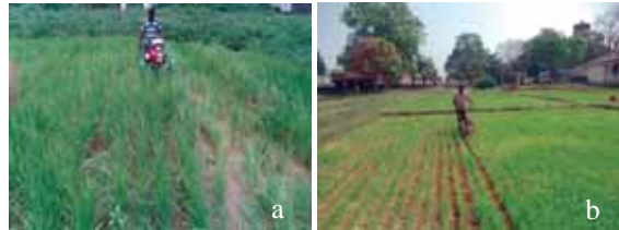
Fig. 5. Weeding in rice with two row wet land weeder (a) and single row dry land weeder (b).
