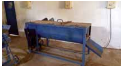
Fig. 4. Mixing unit (Rice Straw + Other ingredients) (Source: IARI, New Delhi)
