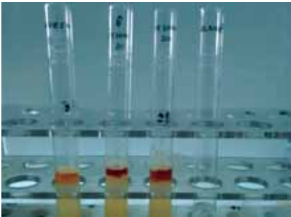
Fig. 1. Rapid color test (xanthoproteic test) to distinguish between low and high protein grains
