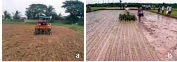
Fig. 4. Tractor drawn seed cum fertilizer drill (a) and self propelled eight row transplanter (b) in operation.
