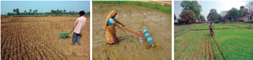
Fig. 9. NRRI developed three row seed drill (a), six row drum seeder (b) and power operated single row dry land weeder (c) in operation.
