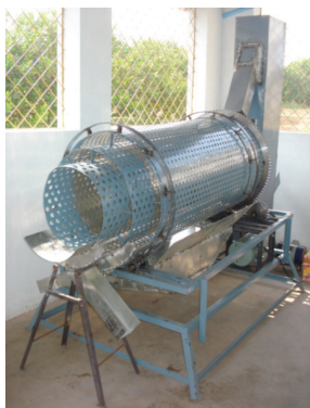
Concentric drum type rotary grader for raw cashewnuts
