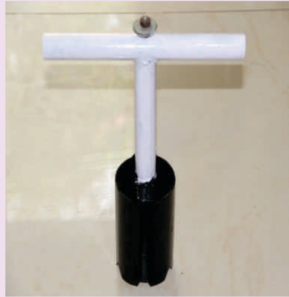
Fig. 14. Prototype of hand held bulb planter
