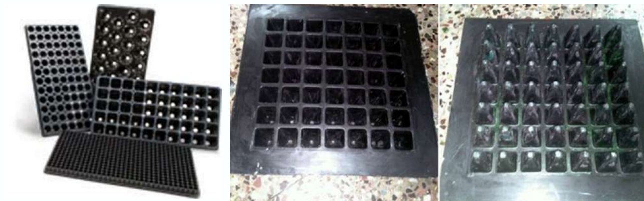
Plastic seedling trays currently used in nursery (left) and the fibre reinforced epoxy mold prepared for preparation of composite based nursery trays (right).
