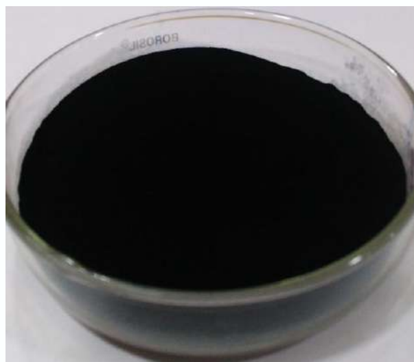
Activated Carbon from Cotton Stalks
