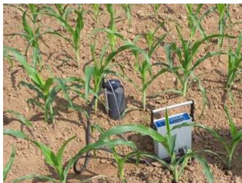
FIGURE 6. Soil respiration chamber and temperature sensor placed on soil
