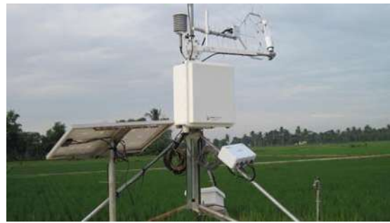
FIGURE 3. Eddy covariance system in rice field
