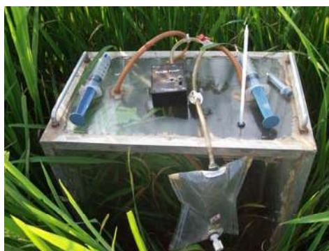
FIGURE 7. Chamber measurement for methane and nitrous oxide emission studies
