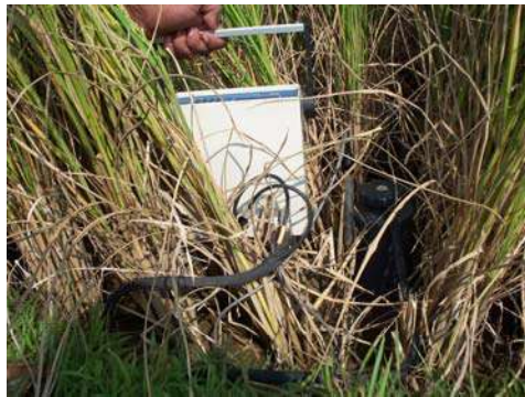
FIGURE 5. Soil respiration chamber in rice field
