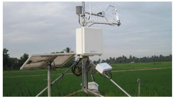
FIGURE 3. Eddy covariance system in rice field
