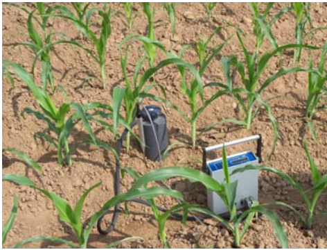
FIGURE 6. Soil respiration chamber and temperature sensor placed on soil
