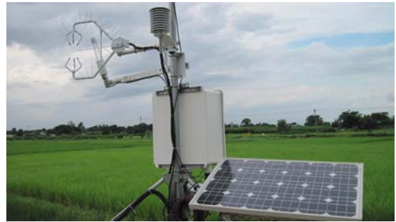
FIGURE 2. Sensors of eddy covariance system
