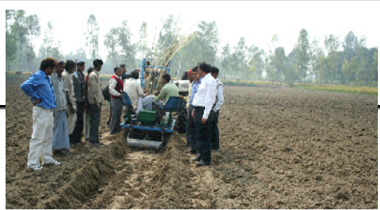
Fig 5.1 IISR tractor operated paired row sugarcane planter in field operation at Sitapur
