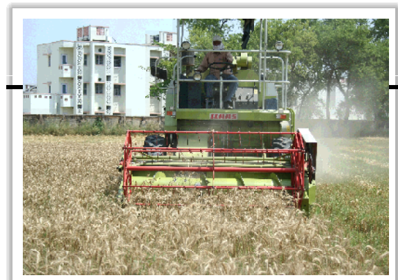
Fig 5.4 Self propelled tangential axial flow (TAF) combine harvester in operation
