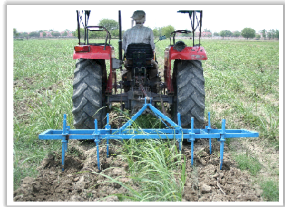
Fig 5.2 Tractor operated interculturing equipment in field operation in wide spaced paired row (30:120 cm) cane crop
