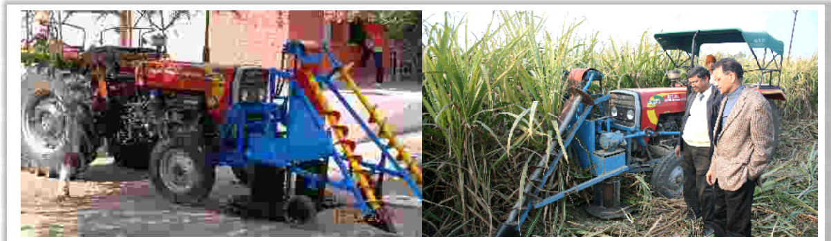
Fig 5.3 Modified tractor operated front mounted sugarcane harvester
