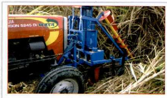
Fig. 5.1. Tractor operated front mounted sugarcane harvester under field operation
