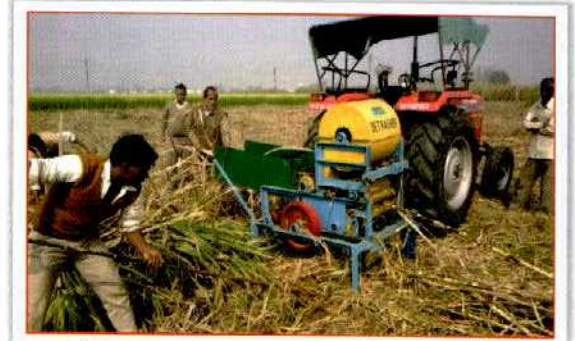
Fig. 5.2. Tractor operated sugarcane detrasher for cleaning of harvested cane
