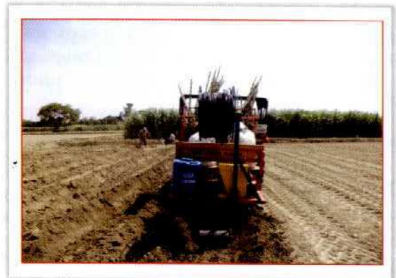
Fig. 5.6. Tractor operated trench planter with sub-surface drip laterals laying attachment
