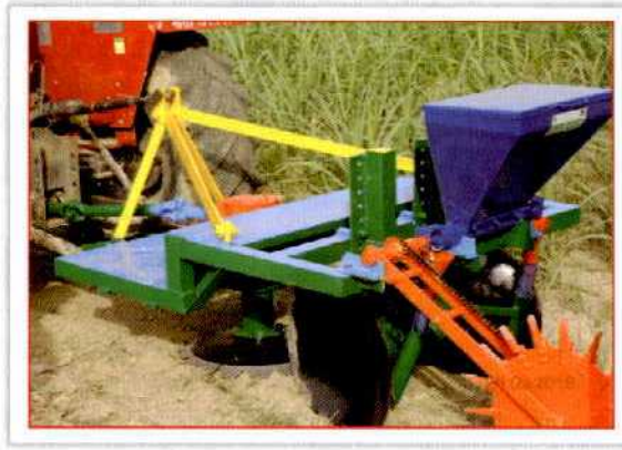
Fig. 5.3. Tractor operated ratoon management device with discs
