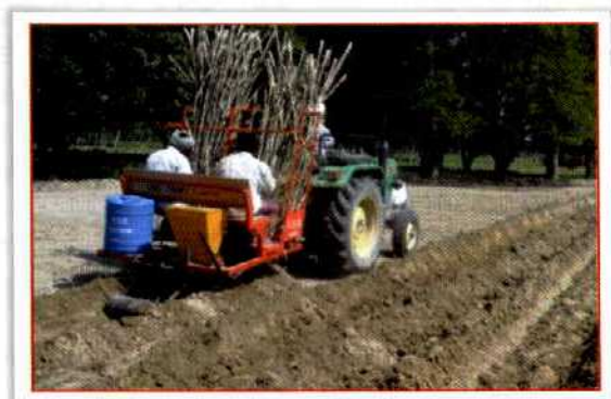
Fig. 5.8. Tractor operated trench planter under field operation at farmer's field in Bakshi-ka-Talab, Lucknow
