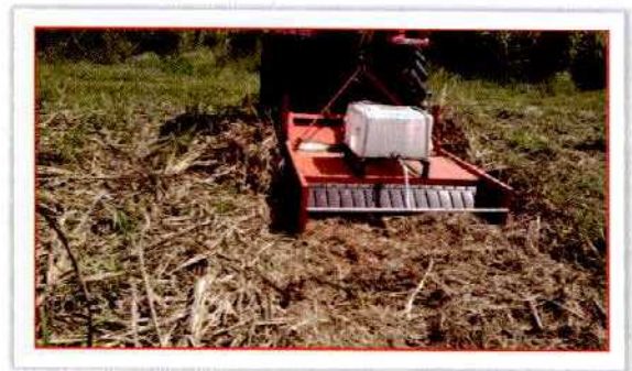
Fig. 5.5. Tractor operated plant residue shredder under field operation
