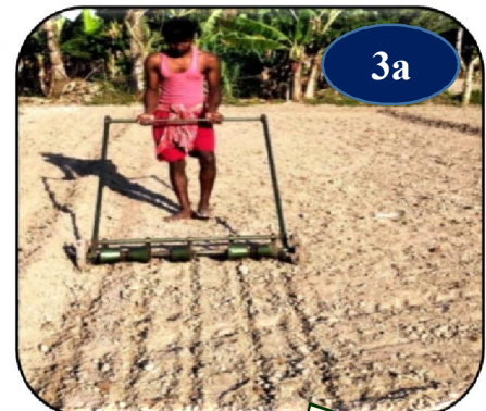
Step-3a: Line sowing of fungicide treated jute seed using CRIJAF Multi-row seed drill
