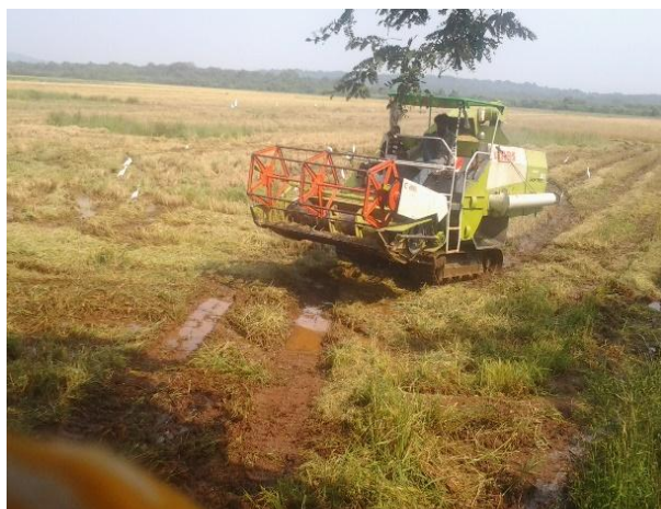
Fig. 3: Harvesting of broadcast sown paddy using combine harvester
