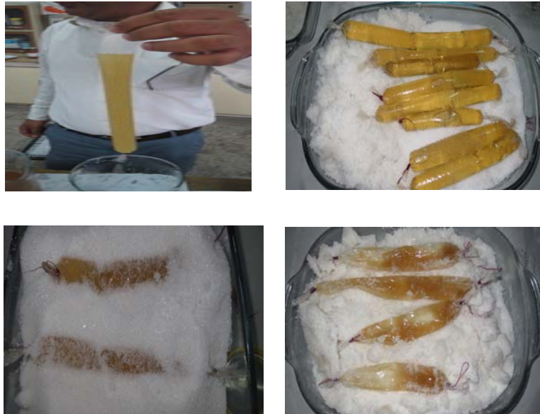
Fig. 4: Osmotic dehydration of excess water through semi-permeable membrane (Molecular weight cut-off range: 12 kDa)
