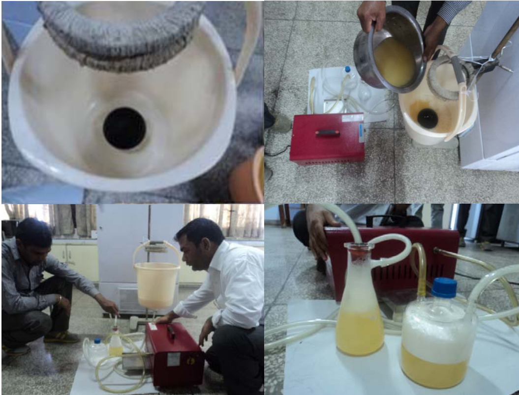
Fig. 7: Set-up of carbon filter and vacuum filtration of kinnow juice
