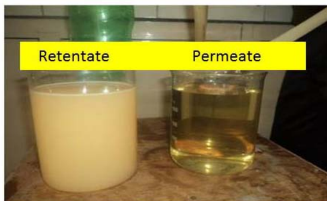
Fig. 6: Ultrafiltration process with permeate and retentate
