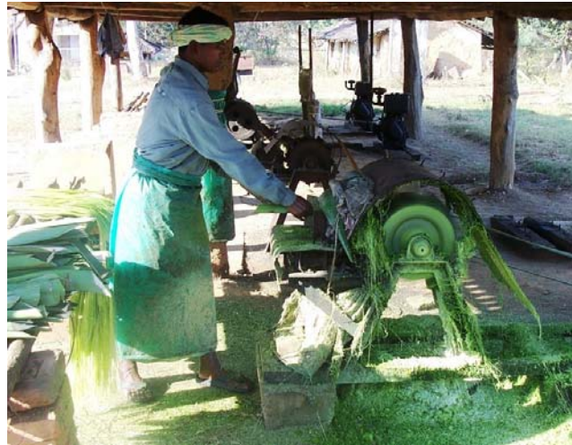
Extraction of sisal fibre using decorticators
