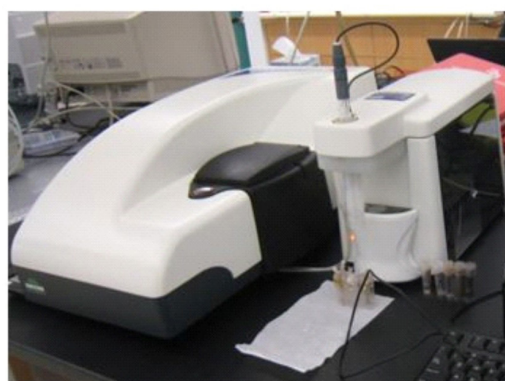
Figure 27.18. Particle Size Analyzer and the principle involved
