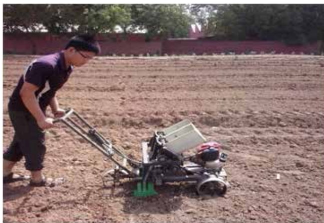
Fig. 5: Field operation of multi-crop planter
