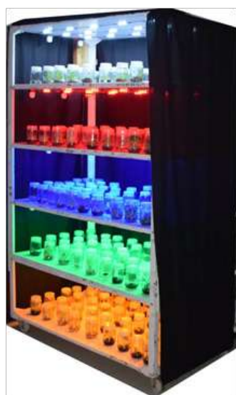
Fig. 8 Culture rack fitted with LEDs of different wavelengths
