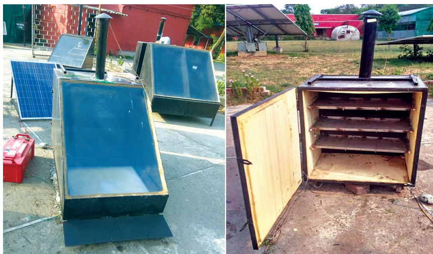
Fig 1 Experimental set up of the dryer.
