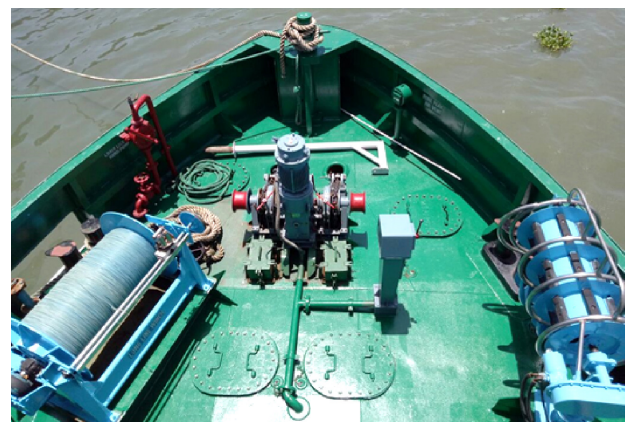
Fig. 4. Main line spooler and three stage gill net hauler on the forward deck of F.V. Sagar Harita
