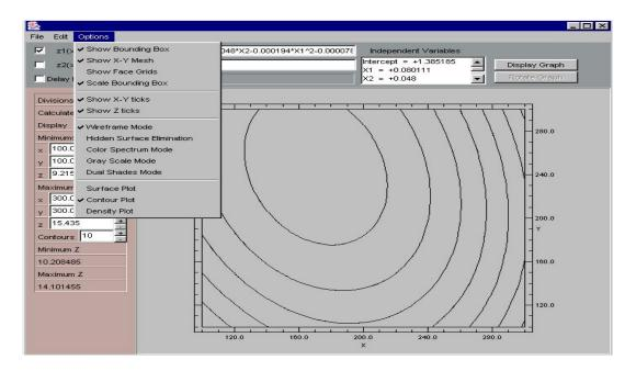
The software is also capable of exploration of the response surface, when the stationary point is a saddle point and lies within the experimental region.
