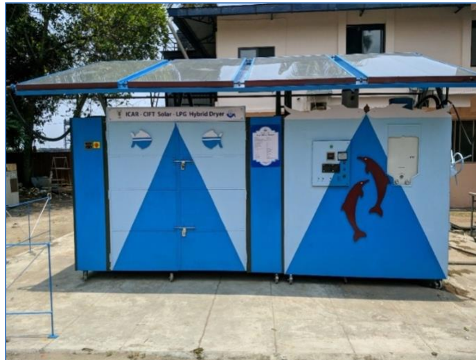
Solar dryer with LPG back up-60 kg
