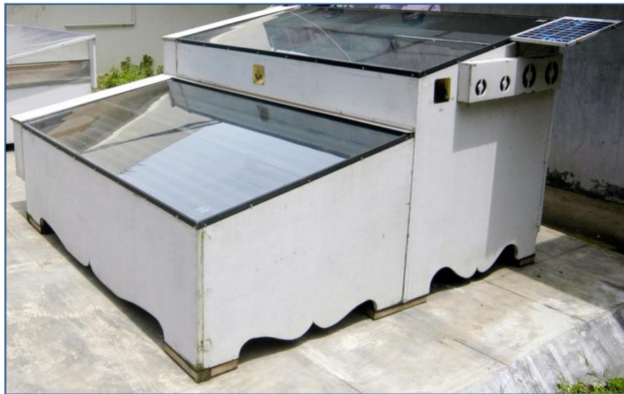
Solar cabinet dryer with electrical back up-40 kg
