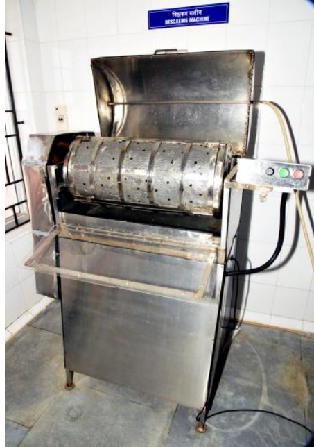
Fig.6 Fish descaling machine with variable drum speed
