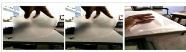
Fig.45. CNF reinforced biofilm from banana starch
