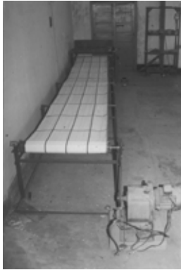
Fig. 1 Test rig for metering of seeds through sticky belt
