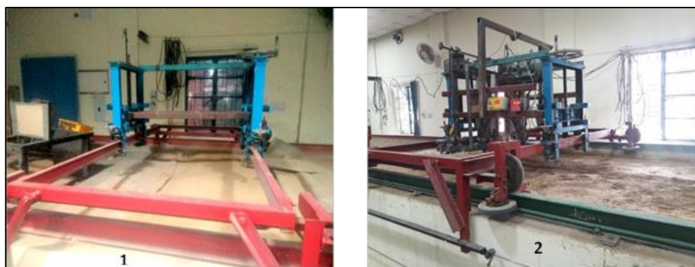
Fig 11: Soil bin before (1) and after (2) mounting the lab test setup for testing tires
