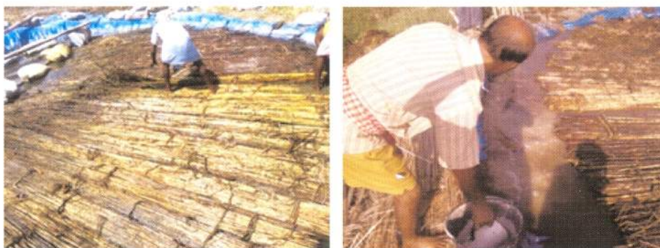
Photo. 14. Jak opening and addition of lime solution along periphery for sanited fibre extraction
