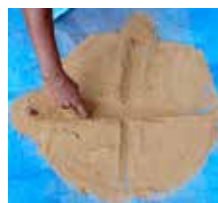
Quartering method of soil sampling
