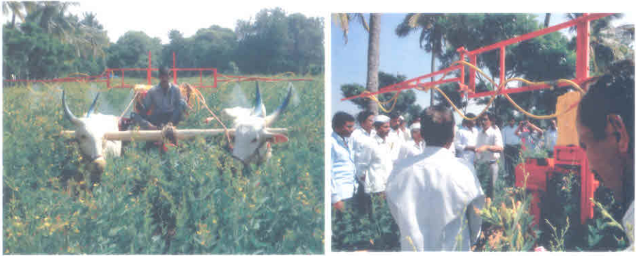
Fig. 2: Demonstration of bullock drawn engine operated sprayer for pigeon pea crop
