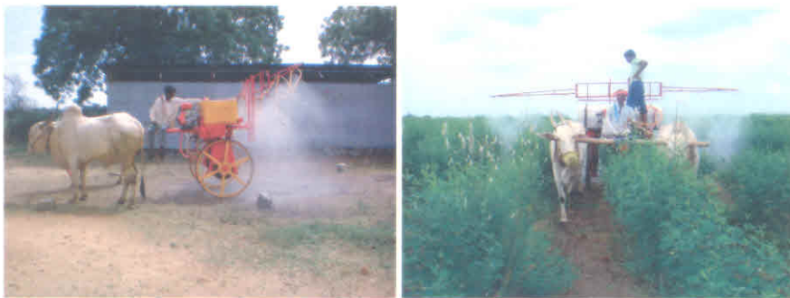
Fig. 1: Functional testing and Working of bullock drawn engine operated sprayer in pigeon pea crop
